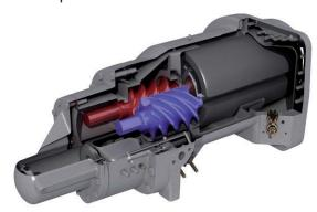
The compressor is driven by a highefficiency motor optimized for watercooled chiller operation. The rotors feature the latest lobe design for R134a operation, running in oversized roller bearings and with variable slide valve capacity control.
